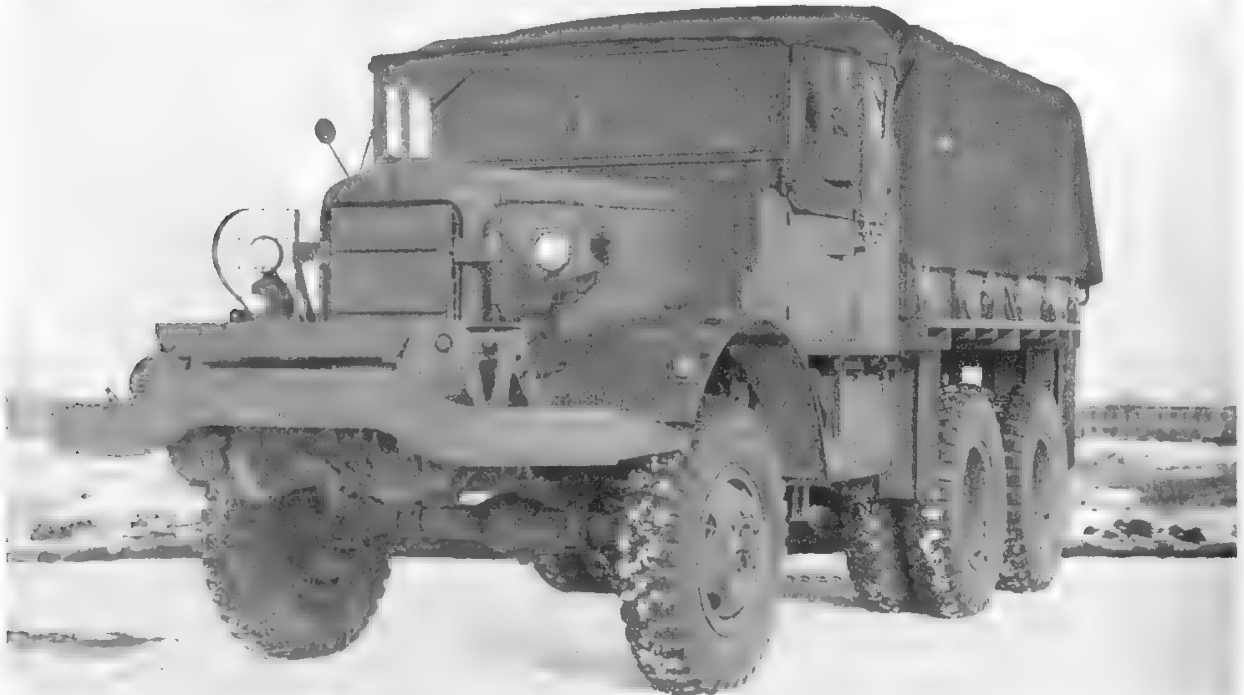
This NO-2 is an example of the first NO production model. The cab and front-end sheet metal were completely redesigned, the steel cargo body has given way to a wooden bed, and a different model of front winch has been used. (Photo courtesy Mack Trucks Historical Museum)
